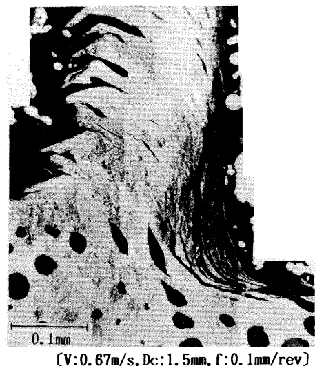
Fig. 7. Chip forming state in machining of FCD1000-2.
