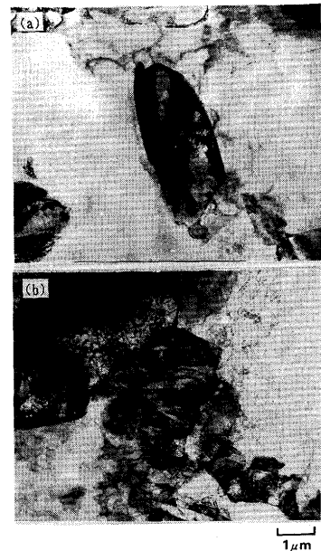
Fig. 2. Examples of the morphologies of retained austenite when the austemper time is 480s. (a) Inside a ferrite (b) On the ferrite boundary
