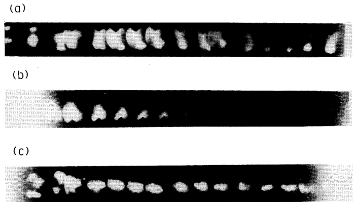
Fig. 5. Time resolved photograph of low voltage discharge of iron under argon atmosphere. (a) discharge with heavy sample vaporization from a spot (concentrated discharge). (b) discharge without sample vaporization (diffuse discharge), (c) discharge with sample vaporization from a few spots (intermediate type).
