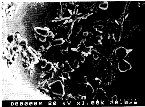
Fig. 13. Inclusions in pinhole.
