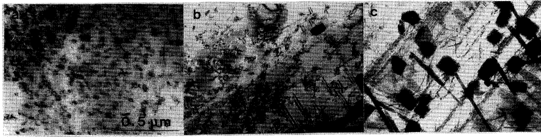
Fig. 2. TEM photographs of A-VT aged at 873K for (a) 3.6 \times 10^3 , (b) 1.08 \times 10^4 and (c) 2.88 \times 10^4 ks. Line marks indicate 0.5 \mu\text{m} .
