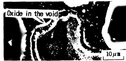
Fig. 9. Morphology of the surface of the substrate of 0.15mm thick Steel B oxidized in air at 1373K for 1800ks.
