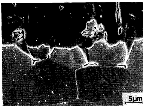
Fig. 7. Penetration of Al-Fe IMC to ferrite grain boundary of steel substrate. (Zn-15 mass% Al coating, Fluxing method, Bath temp.; 520 °C, Immersion time; 5 s)
