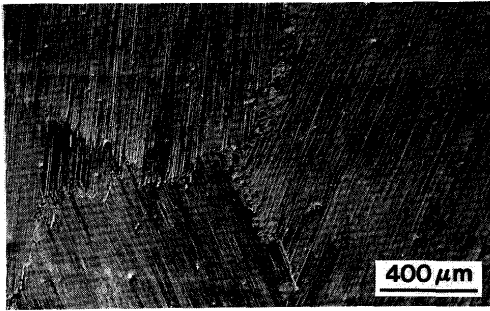
Fig. 3. An optical micrograph of a Ti-48at%Al alloy with the fully lamellared structure. (Courtesy of Prof. M. Takeyama at Tokyo Institute of Technology).
