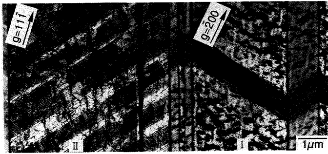
Fig. 4. Deformation substructure of Ti-49.1at%Al PST crystal cyclically deformed ( \phi=0^\circ , \Delta\sigma=430\text{MPa} , N=10^5 , f=1\text{Hz} ).
