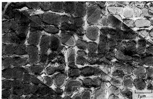
Fig. 10. Transmission electron micrograph of the specimen as heat treated and crept up to minimum creep rate at 1273K-250MPa.
