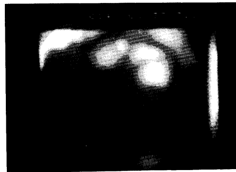
Fig. 14. X-ray fluoroscopic image of bubbles near the bath surface. ( Q_g=79\text{cm}^3/\text{s} , d_{ni}=0.11\text{cm} , d_{no}=0.18\text{cm} )
