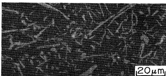
Fig. 1. Optical micrograph of \text{SiC}(w)/\text{Si}_3\text{N}_4 WRC. White acicular grains are \text{SiC}(w) . ( \times 600 )
