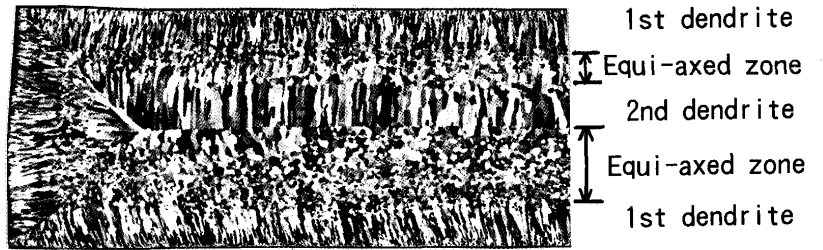
Fig.3 Solidified structure of cast slab stirred by upper EMS in bending CC
