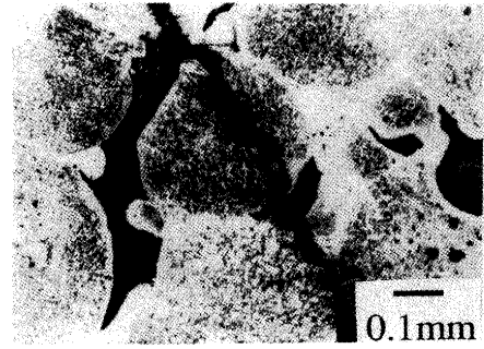
Fig. 6. Enlarged microstructure around circumferential cracks generated with double tube method.
