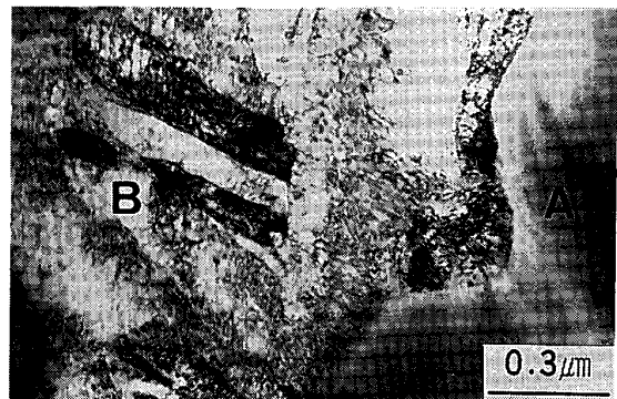
A : \text{Mo}_2\text{FeB}_2 complex boride B : Iron base martensitic binder
