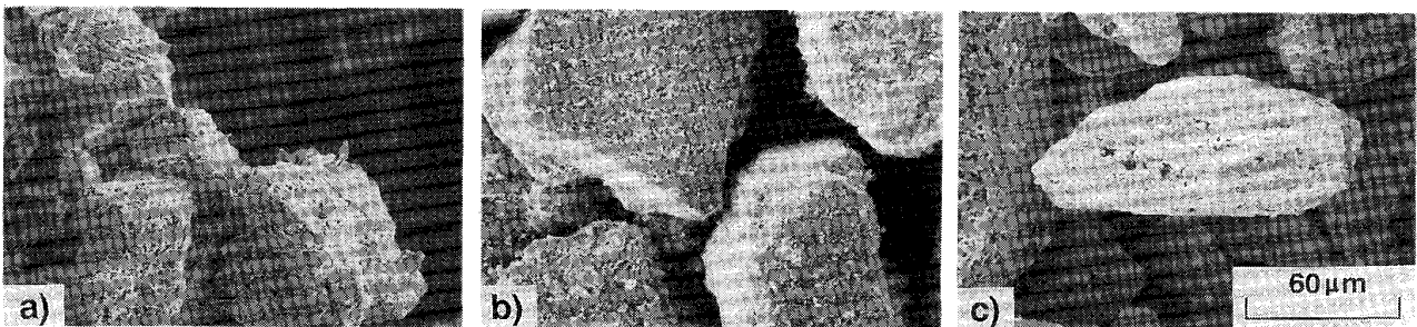
a) Ore A : Sticking at R = 35% (850°C, CO/H 2 = 80/20 vol%) b) Ore F : Non-sticking R = 94% (850°C, CO/H 2 = 80/20 vol%) c) Ore A : Non-sticking R = 26% (900°C, CO/CO 2 = 50/50 vol%) (R : Degree of reduction)
