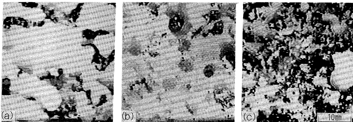
Photo. 3. Pore branch structures of sintering machine (Three-dimensional pore images (a)~(c) are composed by the same method as shown in Photo. 1).
