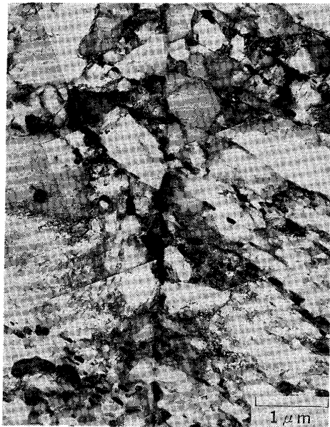
Photo. 2. Transmission electron micrograph of specimen ruptured at 650°C-140MPa, t_r = 935 h.
