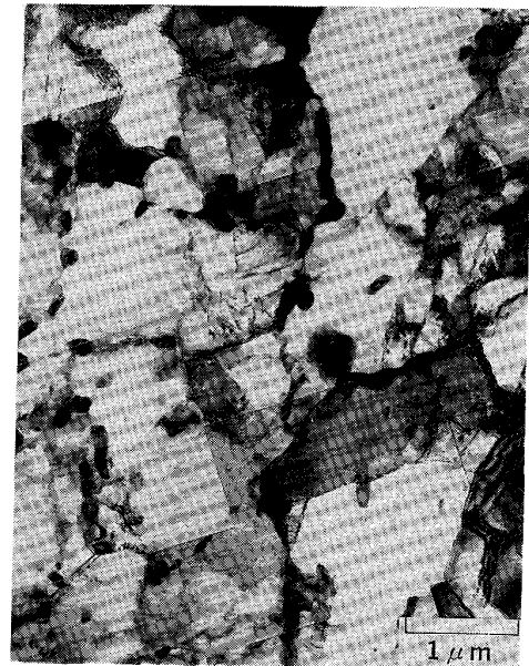
Photo. 3. Transmission electron micrograph of specimen ruptured at 600°C-220MPa, t_r = 2865 h.
