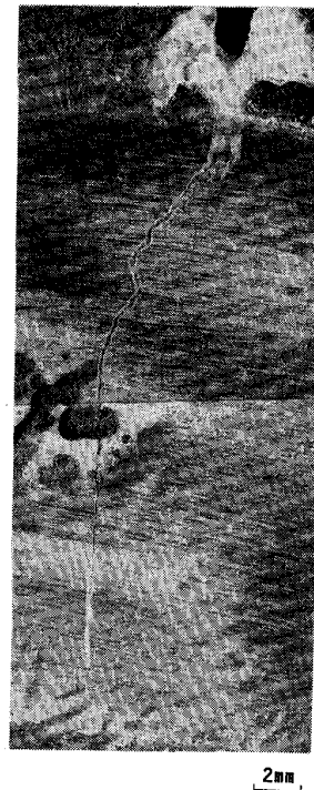
Photo. 3. An example of crack propagation during WOL test.
