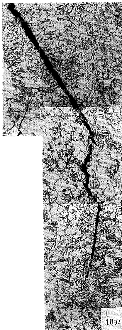
Photo. 5. Crack propagation in dual-phase microstructure.
