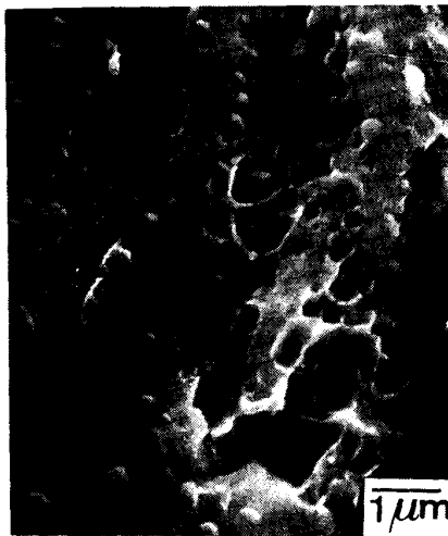
Photo. 4. Voids grown at the grain boundary in the fracture surface after SSC test.
