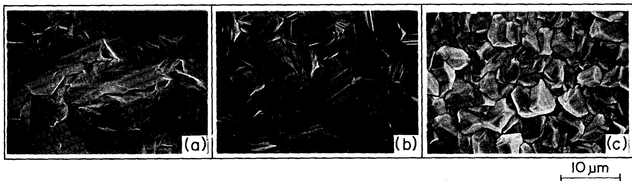
(a) 20A/dm 2 (b) 120A/dm 2 (c) 200A/dm 2 F. R. : 2m/s Photo. 4. SEM micrographs of zinc electrodeposits from chloride bath.
