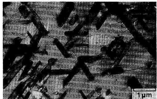
Photo. 8. Transmission electron micrograph of Fe-30Cr-50Ni-2Mo creep interrupted for 308 h at 1023 K-98 MPa. Showing the intragranular precipitation of \alpha' phase.
