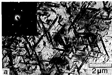
a : Showing the intragranular precipitation of \alpha' phase b : Schematic diffraction pattern of \alpha' phase
