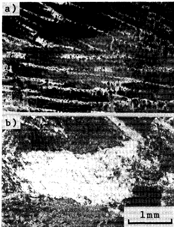
Photo. 3. The comparison between the a) dendritic and b) austenitic structures in 0.2%C steel cooled at 3^{\circ}\text{C}/\text{s} and quenched from 1000^{\circ}\text{C} .
