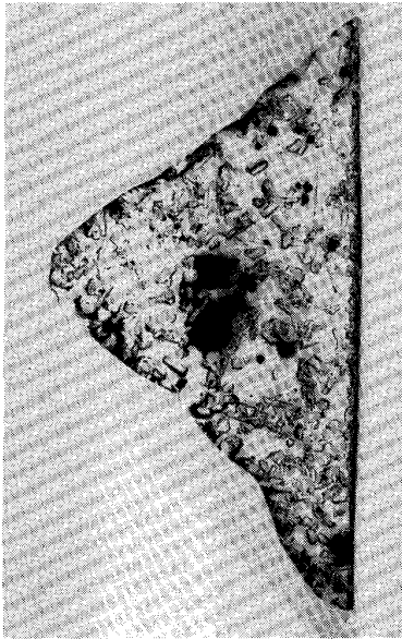
Photo. 1. Microphotograph of reaction product formed at the meniscus of molten metal which was undercooled to 30 K.
