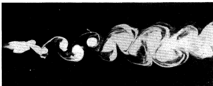
Fig. 2. Separation of boundary layer and formation of vortices.
