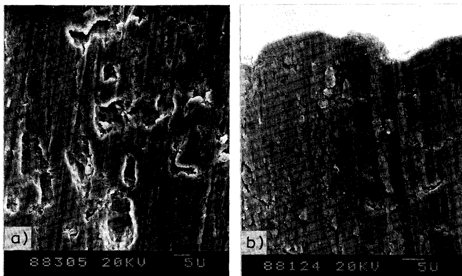
p = 20 MPa \Delta\sigma_a = 150 MPa a) After 10^4 cycles b) After 2.8 \times 10^5 cycles Photo. 4. Fretted surface.
