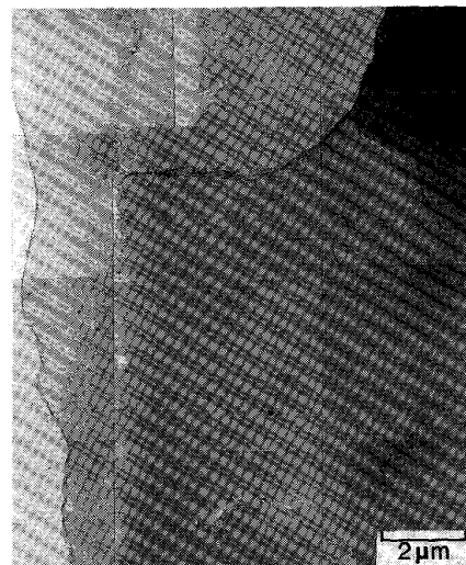
Photo. 2. Transmission electron micrograph of 6Cr crept up to steady state creep stage at 1000°C-3.0 kgf/mm 2 .
