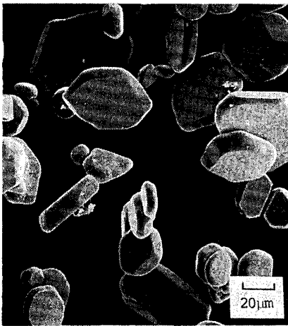
Photo. 1. SEM photograph of \alpha -Fe 2 O 3 crystals grown from Na 2 O·2B 2 O 3 flux.
