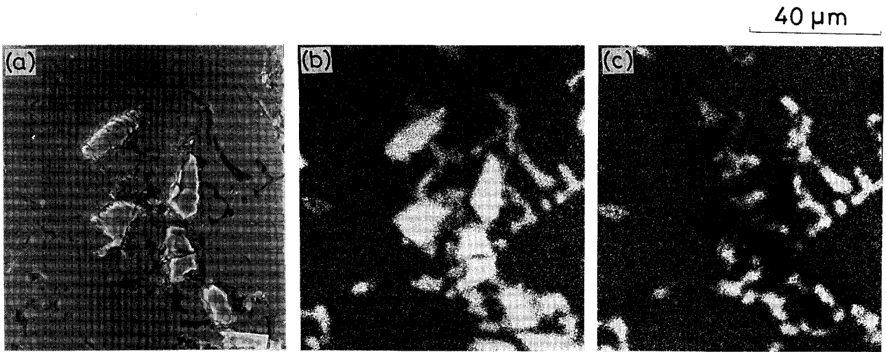
(a) SEM (b) Silicon image (c) Magnesium image Photo. 4. \alpha -SiC particles dispersed in Al-5%Mg alloy.
