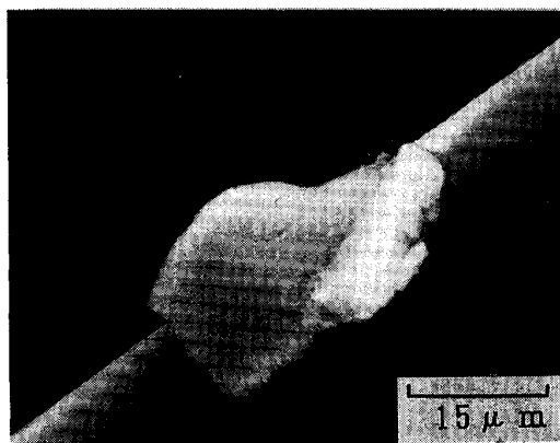
Photo. 5. Scanning electron micrograph of alumina-fiber.
