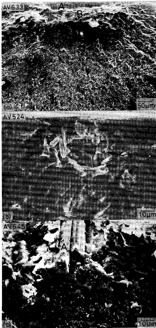
(a) SiC w (10)/A2024 ( \sigma_a = 245 MPa, N_f = 1.17 \times 10^7 ) (b) SiC p (10)/A356 ( \sigma_a = 137 MPa, N_f = 1.01 \times 10^7 ) (c) SiC p (10)/A357 ( \sigma_a = 157 MPa, N_f = 2.03 \times 10^6 )
