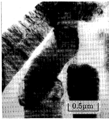
Photo. 2. TEM micrograph of 20%SiC w /6061-T6 composite consolidated at 660°C.
