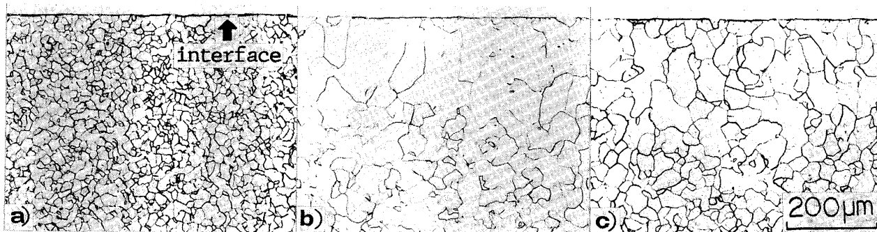
a) As hot rolled b) Annealed at 950°C c) Annealed at 1050°C
