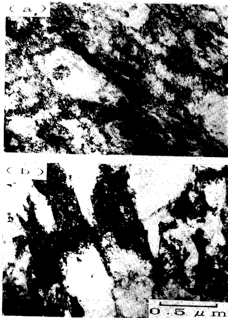
Photo. 3. Transmission electron micrographs of (a) 16Cr-9Ni-0.1C steel annealed at 923 K for 3s and (b) 16Cr-10Ni steel annealed at 923K for 10s after 90% cold rolling. Samples were aged at 290K for 60 ks over after annealing, showing cell structure in recovery process.
