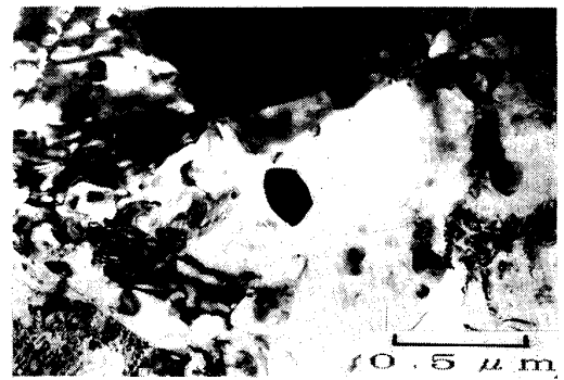
Photo. 4. Transmission electron micrograph of 16Cr-9Ni-0.1C steel annealed at 923K for 60ks after 90% cold rolling. Sample was aged at 290K for 60 ks after annealing.
