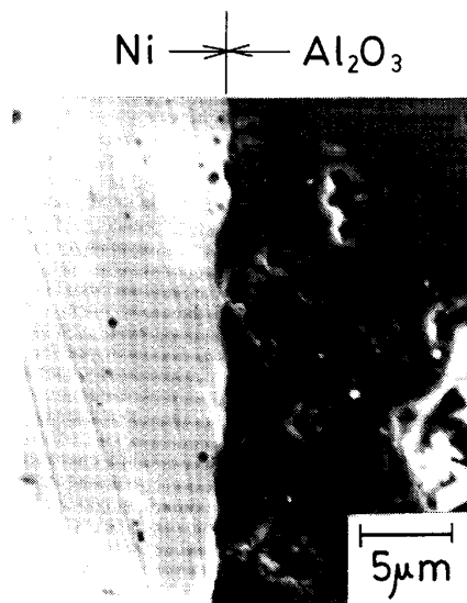
Photo. 5. SEM observation at the interface between Ni and \text{Al}_2\text{O}_3 kept for 7.2 ks in Ar atmosphere.
