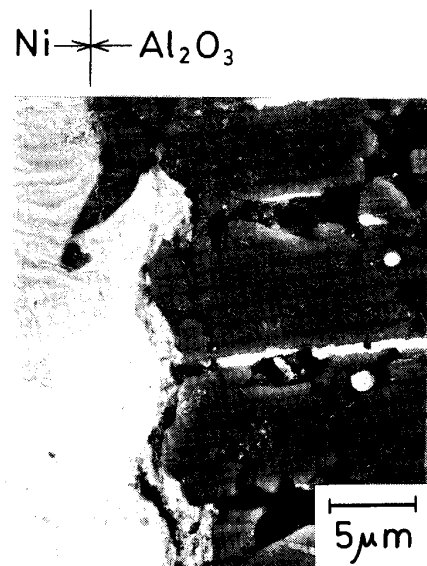
Photo. 3. SEM observation at the interface between Ni and Al 2 O 3 kept for 360 ks in H 2 atmosphere.
