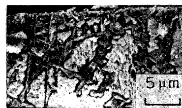
Photo. 1. Oxide penetration observed in a Pt-Rh limb used at 600°C for 120 000 h (SEM).
