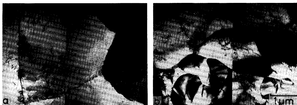
Photo. 5. Transmission electron micrographs near grain boundary of C1 (a) and C2 (b) interrupted the creep test at steady state stage ( \epsilon=10.5\% ) at 850^{\circ}\text{C} - 39.2\text{ MPa} .
