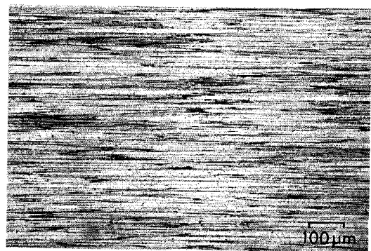
Photo. 2. A microstructure of longitudinal section of specimen BN-2 as heat-treated at 1260°C for 1 h.
