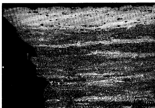
Photo. 3. A microstructure of longitudinal section of the fractured part of BN-2-1 after 3 500 h under the creep condition of 1 050°C, 16 kgf/mm 2 . Stress-axis is horizontal.
