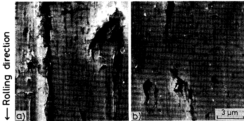
Photo. 1. Scanning electron micrographs of wear surfaces of a) 1%C-0.08%V (steel A) after 7 \times 10^6 cycles and b) 1%C-1.0%V (steel B) after 1.2 \times 10^7 cycles tested under the condition of high Hertz stress ( 200 \text{ kgf/mm}^2 ) and low slip ratio (9%).
