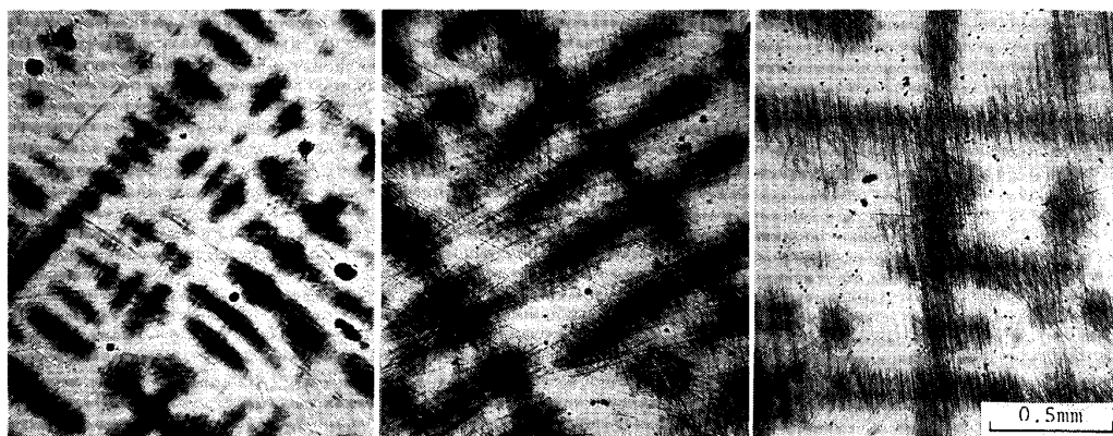
(1250°C × 8h) (1250°C × 16h) (1250°C × 24h) Photo. 3. Transformation of microstructure by heat treatment.
