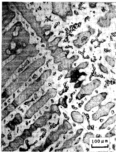
Photo. 2. Solidification structure (5°C/min).
