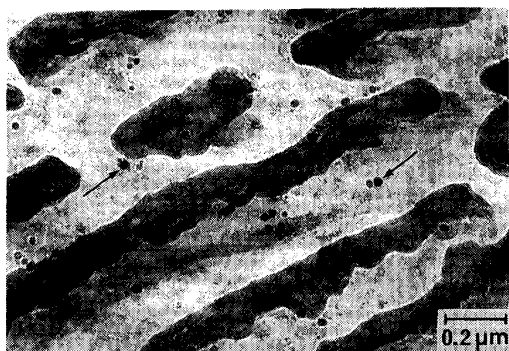
Photo. 7. Extraction replica image of a Steel B specimen deformed at 650°C at \dot{\epsilon} = 0.83 \times 10^{-3} \text{s}^{-1} , showing V(C, N) precipitation within the matrix. Dark areas are due to lamellar precipitation of cementite formed during cooling from the deformation temperature.
