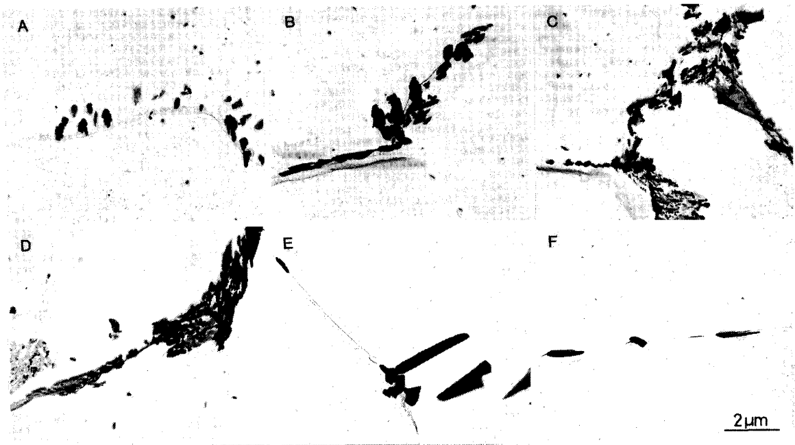
Photo. 2. Extracted replicas from the steels aged at 973 K for 720 ks.
