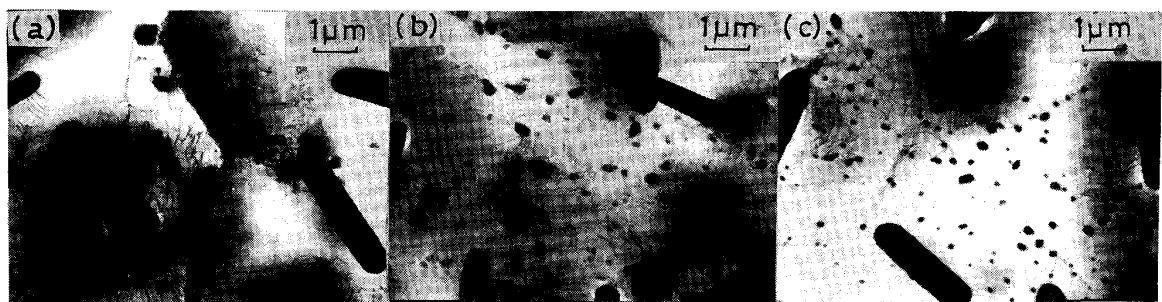
Photo. 6. Characteristic X-ray images of 1402 ruptured after 2508 h at 1000°C in air.
