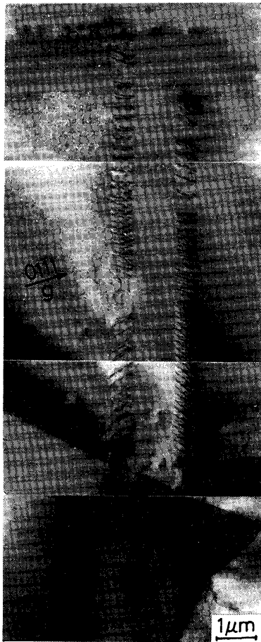
Photo. 4. Dislocation arrays on prism planes for a sample deformed at 4 K which pass through grain boundaries (region II : stress amplitude = 1365 MPa, N_f = 14\,437 cycles). Foil cut from hour-glass type specimen.
