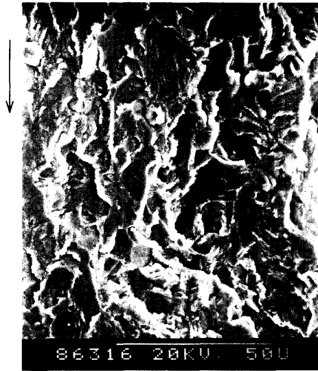
Sea water, \Delta K = 9 \text{ kgf/mm}^{3/2} , R = 0.77 Photo. 6. Fractograph of specimen SL.
