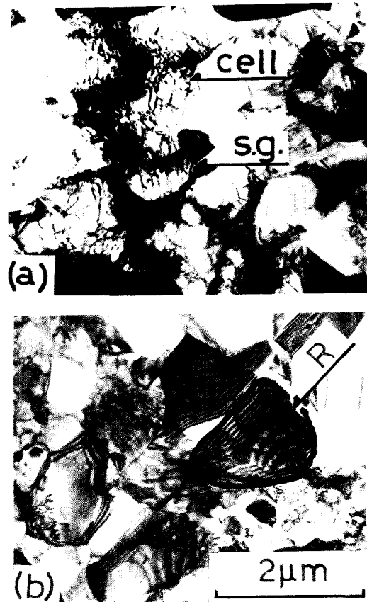
Photo. 3. Transmission electron micrographs of 16-10 steel annealed at 923 K for 0.6 ks after 90% cold rolling: Showing dislocation cell, subgrain (s.g.) and recrystallized austenite (R). Both (a) and (b) were obtained from different area in the same specimen.
