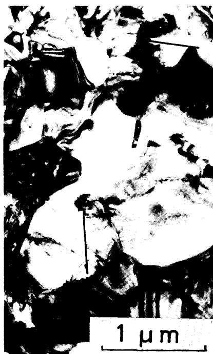
Photo. 3. Transmission electron micrograph of a 15.6%Cr-9.8%Ni stainless steel annealed at 873 K for 0.6 ks after 90% cold rollings. Arrows show subgrain boundaries.
