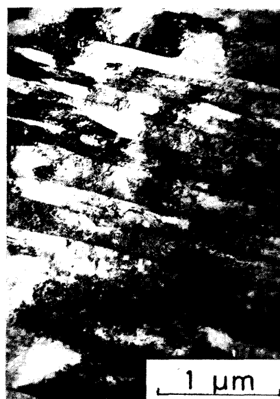
Photo. 1. Transmission electron micrograph of a 15.6%Cr-9.8%Ni stainless steel with 16% cold rolling. Showing lath martensite induced by cold rolling.
