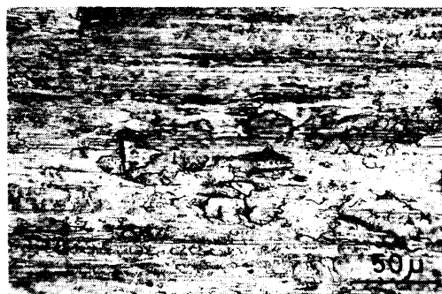
Photo. 3. Optical micrographs of cold rolled surface of steel sheet with roughness of 46\mu\text{m} in H_{max} after annealing and pickling.
