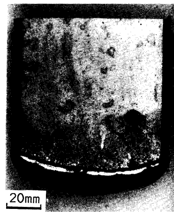
Photo. 2. Solid electrode after melting.
